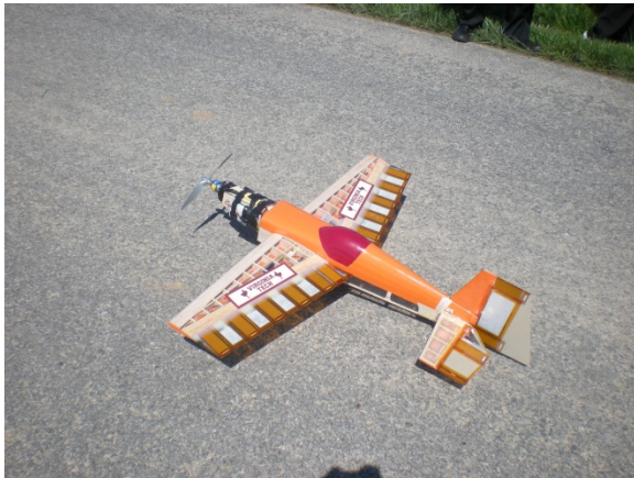
Virginia Tech Wing Morphing Design 2009-2010 Team Aircraft with all solid-state MFC actuated control surfaces. The picture is taken before first flight on April 29, 2010 in Kentland Farm, Blacksburg, Virginia.
