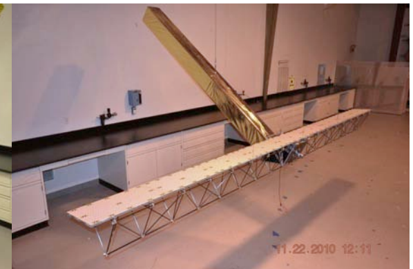
5m x 0.2m Ka-band radar panel demonstration, stowed and deployed.
