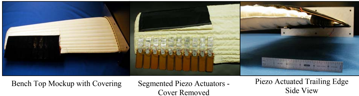
Figure 11 – Trailing Edge Deflection Morphing Wing Prototype
