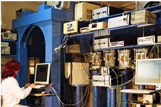
Fig. 7: The experimental set up for resonant testing of four PZT patches bonded on steel beams.
