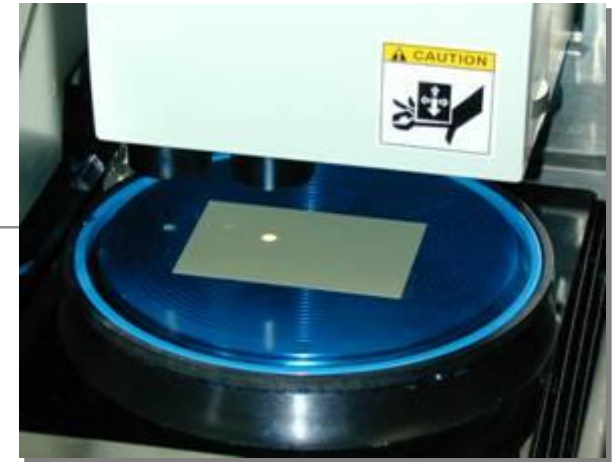
2. Wafer and grip-tape frame positioned for dicing
